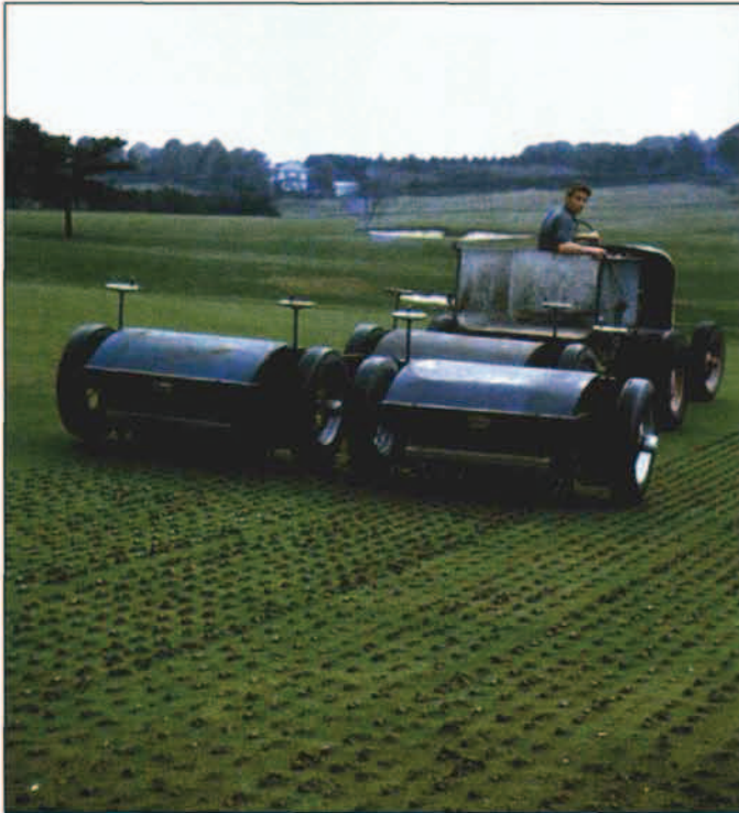
Aerification has been a part of turf maintenance for a long time. This West Point Aerifier was patented in 1946.
