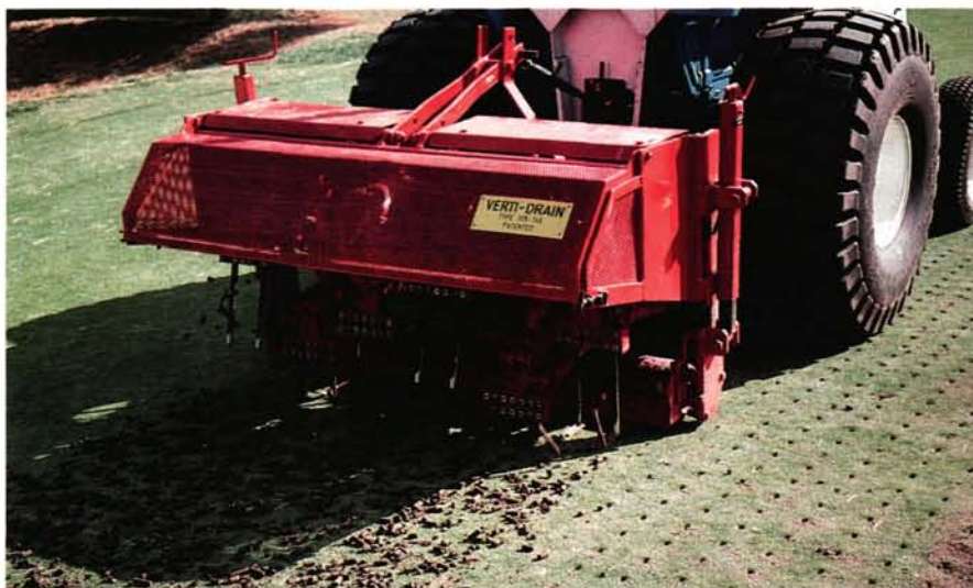
(Top) Floyd-McKay drill aerator, 1987.
