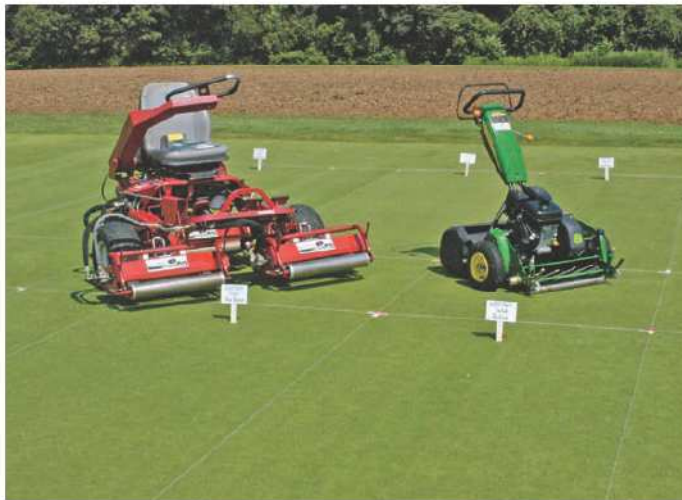
Lightweight vibratory rolling (left) and mowing practices (right) were tested to determine their effect on anthracnose and putting green speed.
