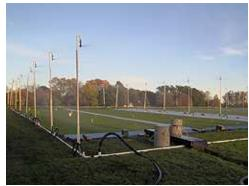
At the University of Minnesota Turf Research, Outreach, and Education Center in St. Paul, Minnesota, a rainfall simulator is used to generate runoff. Plots were equipped with rain gauges and automated runoff samplers to measure precipitation, runoff, and flow rates, and to collect periodic runoff samples. (D2561-1)
