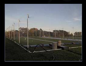
At the University of Minnesota Turf Research, Outreach, and Education Center in Saint Paul, Minnesota, a rainfall simulator is used to generate RUN-OFF. Plots were equipped with rain gauges and automated RUN-OFF samplers to measure precipitation, RUN-OFF, and flow rates, and to collect periodic RUN-OFF samples.
