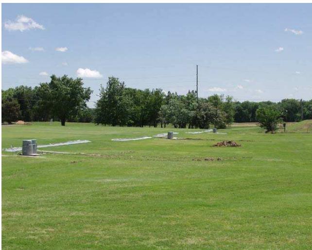
The water runoff research site at Oklahoma State University consisted of three irrigation blocks with two 40 by 80 ft. plots per block for a total of six plots on 0.44 acres.
